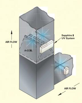
Depiction of an upblast cooling coil set up with a Sapphire Model SA2 mounted above the coil and a Sapphire Model SA1 mounted in the cool air return duct.
