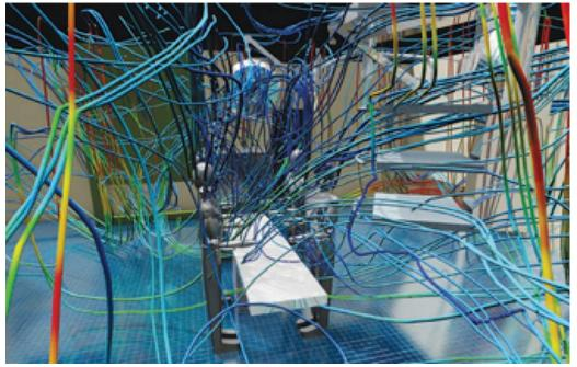
The sample illustration shows a CFD (Computational Fluid Dynamic) model of the air flow patterns in a typical OR.
