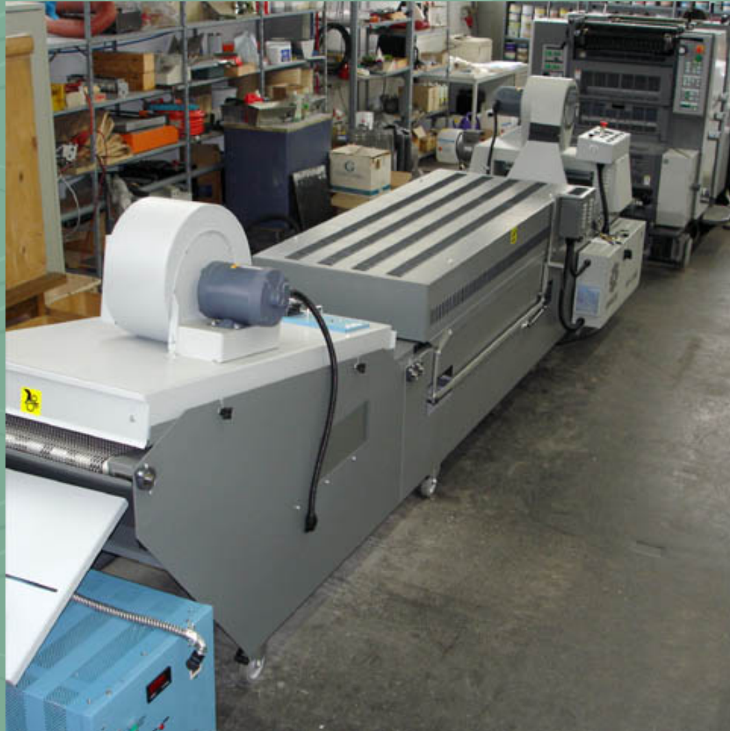
The HP-20 in line to a 2-colour offset. Please also note the UV unit (blue) under the Sunrise sheets delivery.
