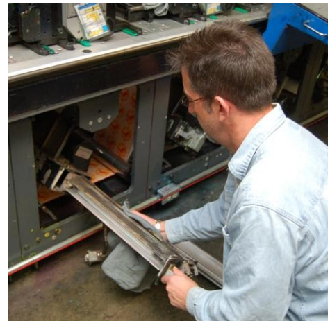
Changing an AUV Ultrapack® UV module is as quick and simple as changing a toner cartridge on a printer.
