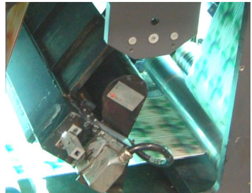
High-output, highly focused UV curing stations provide Hub Labels with better print quality and fewer problems than conventional print
