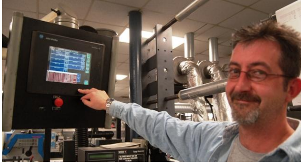
Centralized UV lamp controls make it easy for technicians to quickly fine-tune the output of each curing station to achieve the perfect results.
