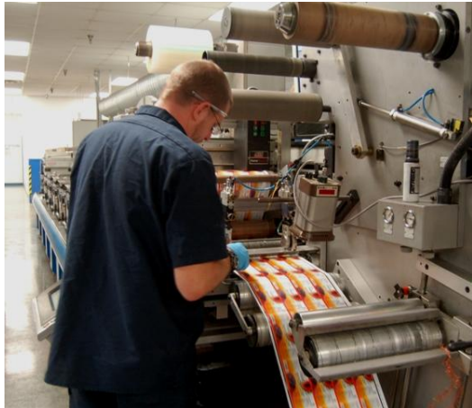
A Hub Labels operator inspects print quality at the end of a multi-stage UV curing Gallus Press equipped with American Ultraviolet UV lamps.
