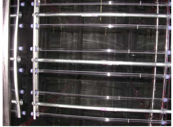
Figure 2-2. Device installed inside the test rig. There are six lamps and three support rods.
